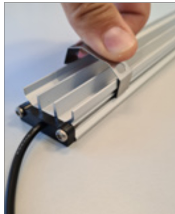
Fig. 3: Spread the suspension bracket slightly so that it protrudes over the cooling fins on the opposite side of the FLEX II.
